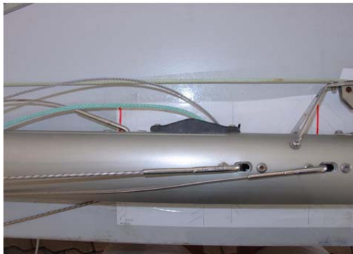
Rigging points: shroud, forestay, trapeze. Heights to be measured from MDP.
