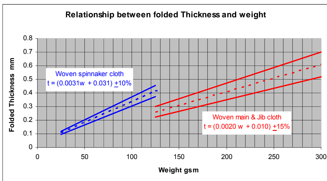
Figure K.1.2.2 Woven ply thickness vs. weight
