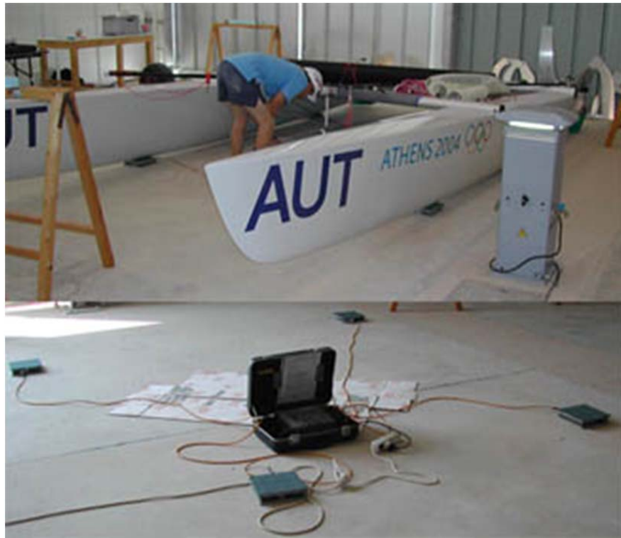
Figure F.7.1.9 Tornado weighing using a 4-pad scale.
