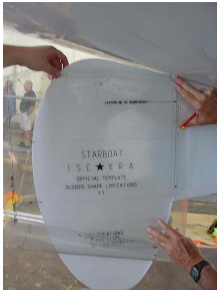
Figure I.5.4 Profile check with mylar template.
