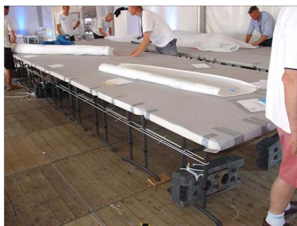
Figure K.3.2 Sail measurement table
