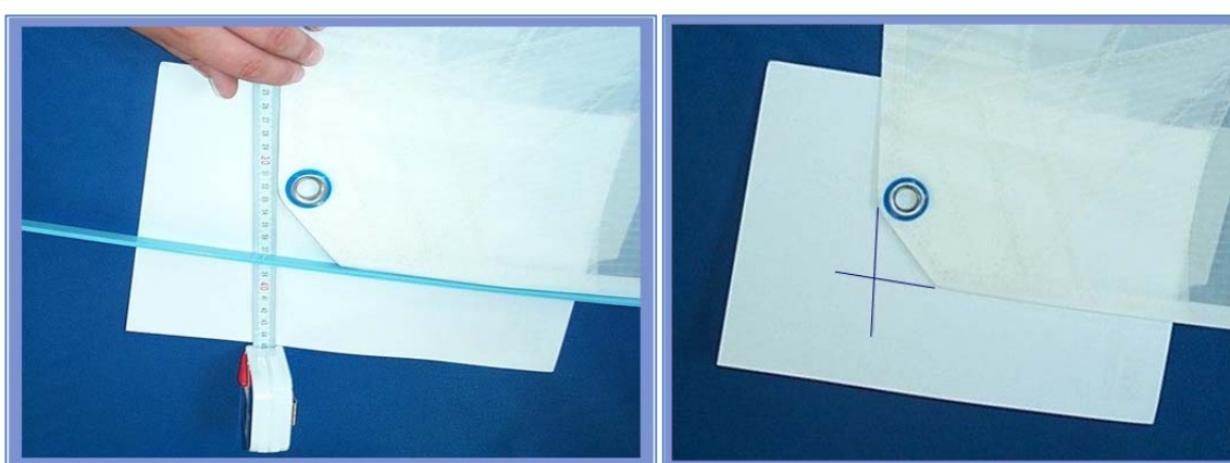
Figure K.2.1.2 Clew point marked on paper.
