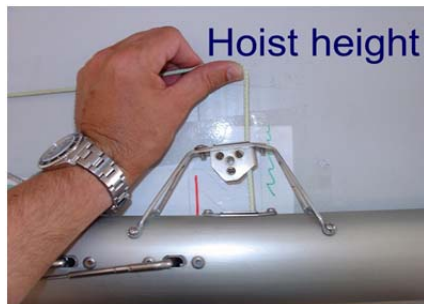
Spinnaker hoist height with the halyard at 90° to the spar.
