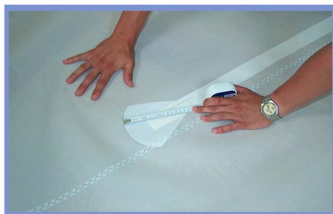
Figure K.2.4.3 Batten pocket patch size.
