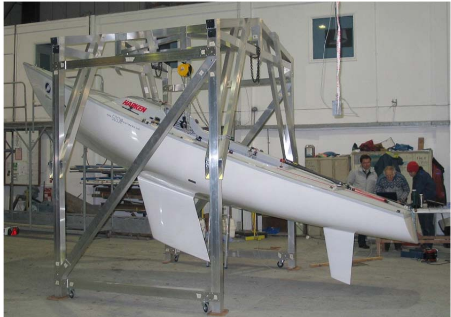
Figure H.4.7.3 An Yngling undergoing a tilt test
