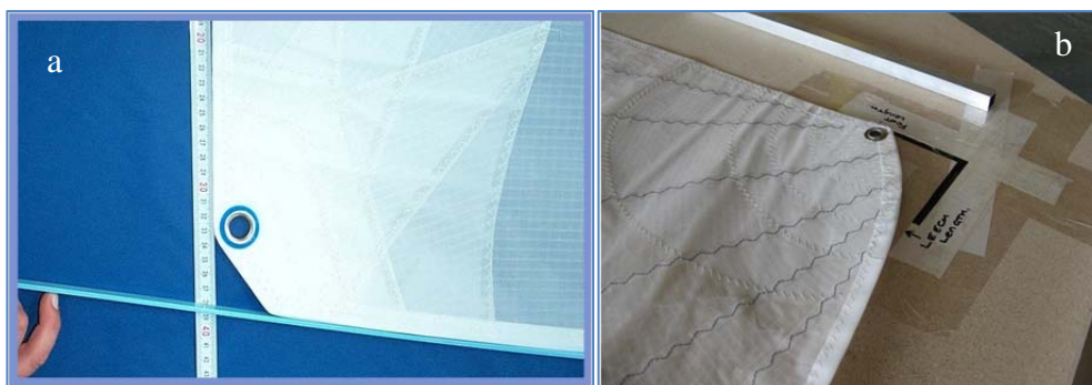
Figure K.2.1.1 Clew point definition.
