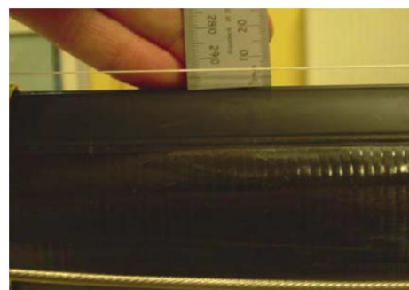
Mast spar curvature and deflection tests: Measurement without load (left) and with load (right).
