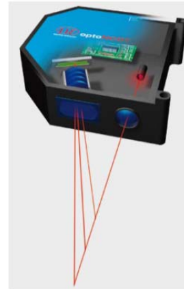
Figure F.6.2.2 A laser triangulation sensor
