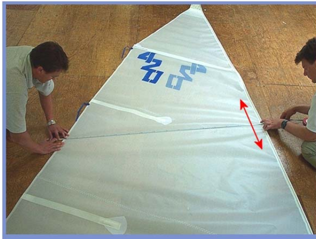
Figure K.2.3.8 Mainsail half width.
